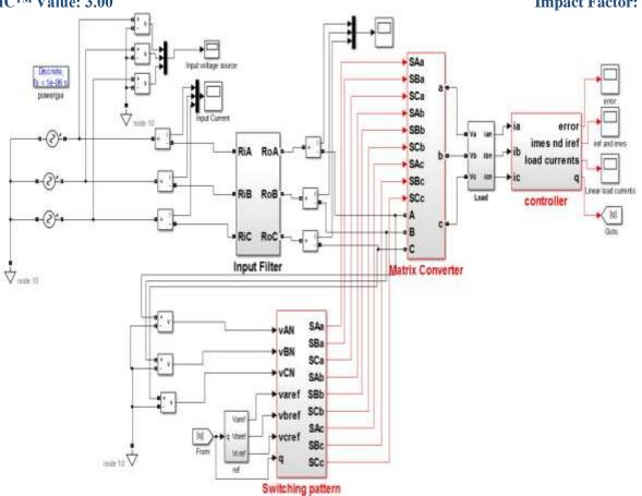
Fig 4.1: Simulink Model Of Controllers Fed To Matrix Converter
