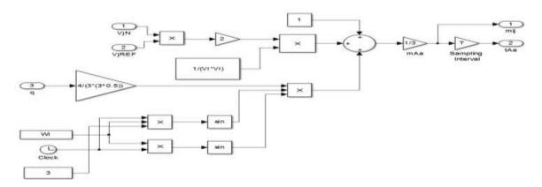
Fig 2.3: Simulink model of matrix converter to generate duty cycle for one output phase
