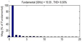
Fig 5.2 : Harmonic spectrum analysis of linear load current (PI controller)
