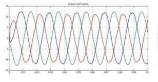
Fig. 5.3: Linear load current (Fuzzy Logic Controller)
