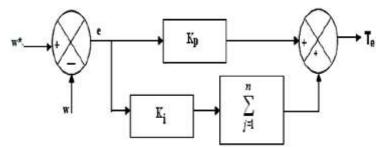
Fig 3.1: Block diagram of PI controller
